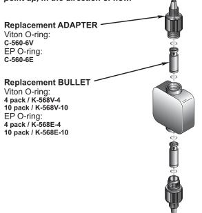
**NOTE:** wear eye protection when working on your pump as discharge lines are under pressure.
