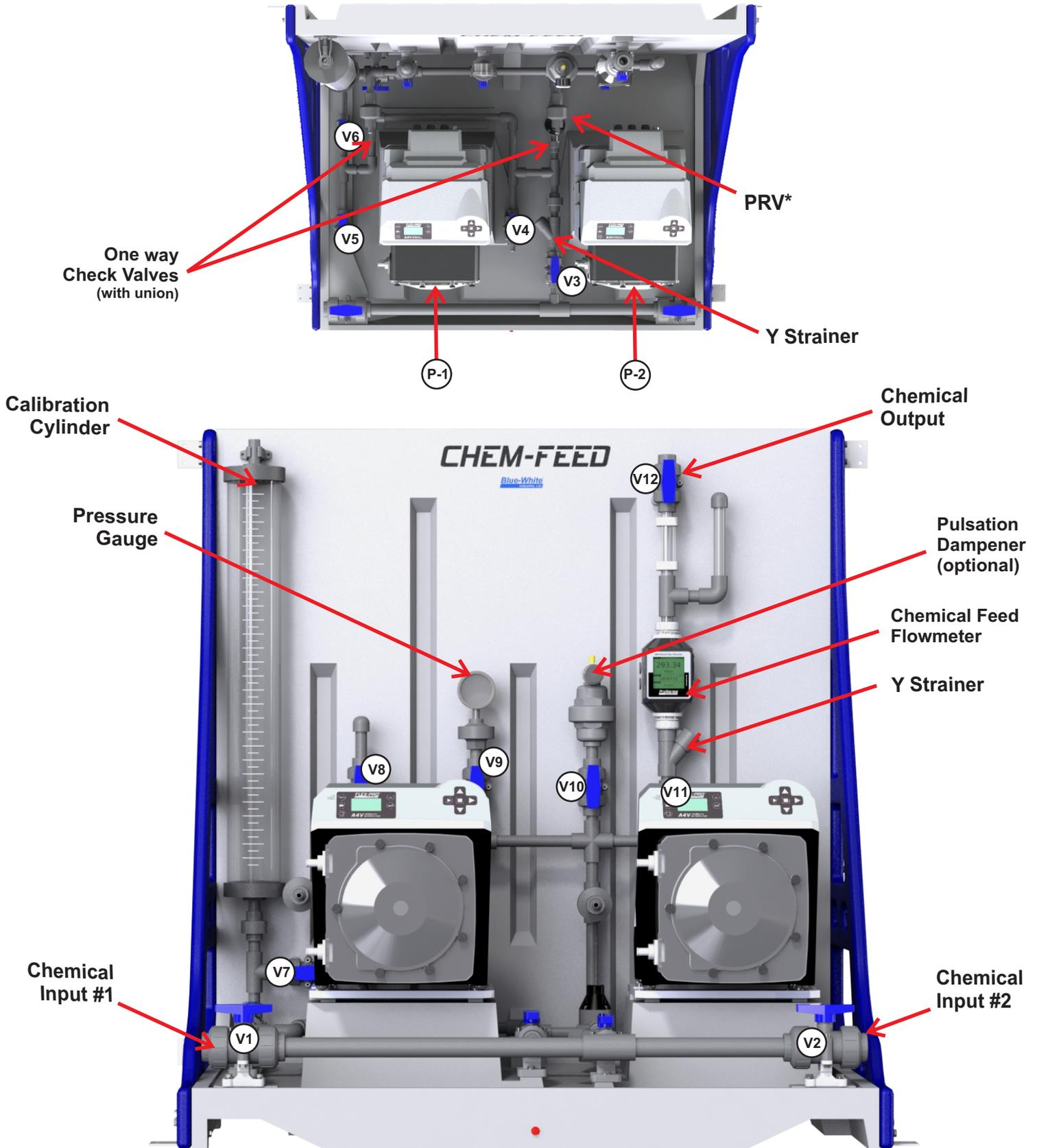
\* PRV = Pressure Relief Valve preset at 50psi
