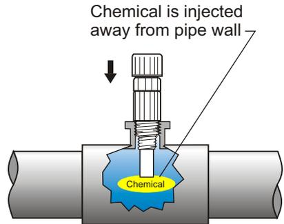
You can install the Injection Fitting directly into your pipe.
