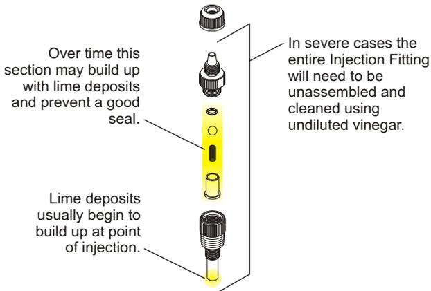
**Optional Threaded Injection Fitting (check Valve) installation.**
