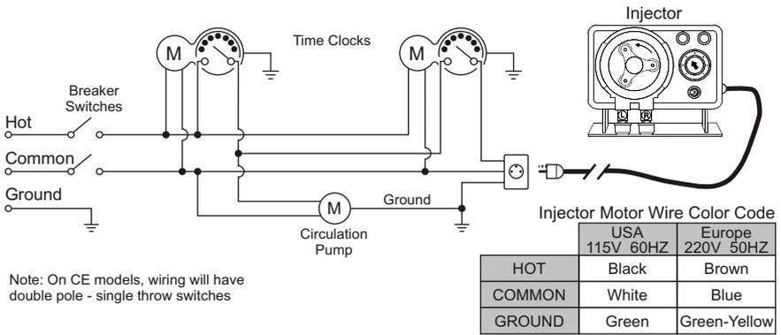
Note: On CE models, wiring will have double pole - single throw switches
