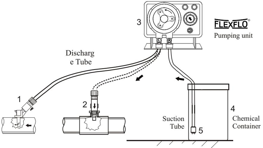
1. The threadless injector requires 3/8" DIA. Hole only.
