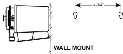
Note: For wall-mounting, recommend drill & thread into solid wood only.
