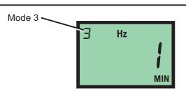
**Time-out** - CHEM-FEED® pumps have a time-out setting of approximately 20 seconds while in configuration menu. If built-in timer exceeds 20 seconds without a button being pressed, then pump will exit configuration menu. Changes will automatically be saved if programming mode is allowed to Time-Out.
