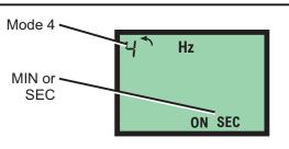
**Time-out** - CHEM-FEED® pumps have a time-out setting of approximately 20 seconds while in configuration menu. If built-in timer exceeds 20 seconds without a button being pressed, then pump will exit configuration menu. Changes will automatically be saved if programming mode is allowed to Time-Out.
