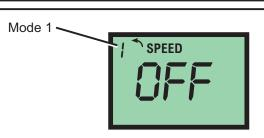
With pump operating in manual mode (Mode 1), pump speed can be changed at anytime by using UP or DOWN arrows during operation.
