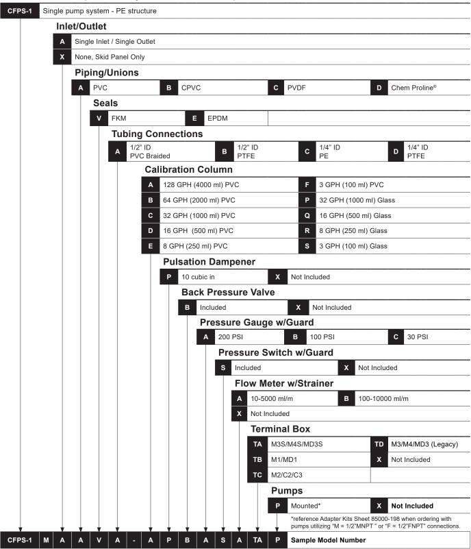
**NOTE:** When ordering pumps for skids, pump head orientation is standard LEFT facing only. All skids are pressure tested prior to shipment. Pumps are purchased and shipped separately. Contact factory for quote/pricing on 5-point performance testing.
