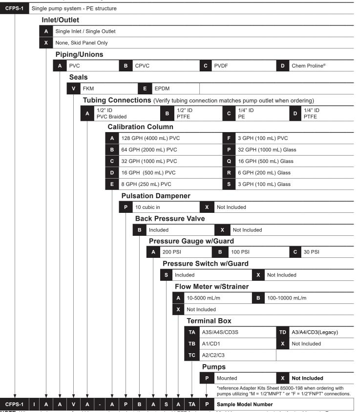
**NOTE:** When ordering pumps for skids, pump head orientation is standard LEFT facing only. All skids are pressure tested prior to shipment. Pumps are purchased and shipped separately. Contact factory for quote/pricing on 5-point performance testing. **Customer is responsible for ensuring skid components are compatible with any chemicals being used.**
