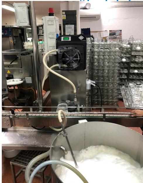
The company was previously using a Pulse Batch feature in their production line. The application was for dosing a predetermined amount of “nutrient-water” into a glass jar, where the small sprig of a fruit tree, almond tree...would begin the growth/germination for eventual planting in the field.
