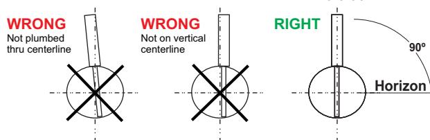
**Note:** Incorrect installation may result in a damaged pitot tube.
