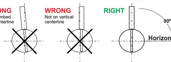
**Note:** Incorrect installation may result in a damaged pitot tube.
