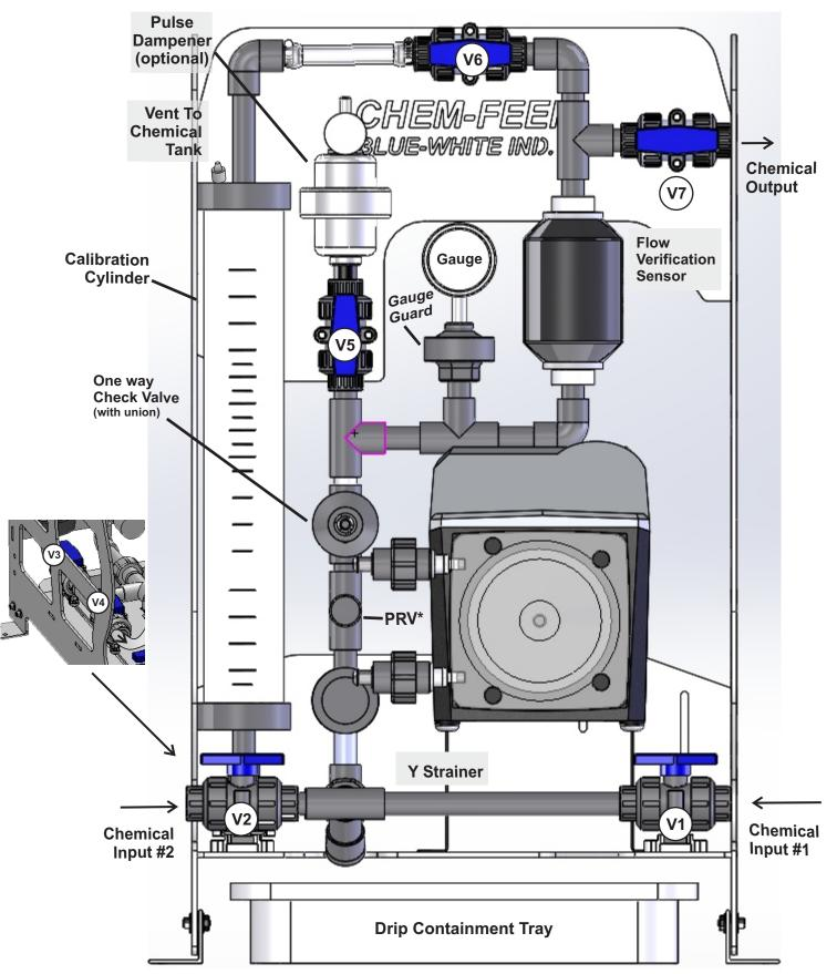
\* PRV = Pressure Relief Valve preset at 50% maximum gauge rating.
