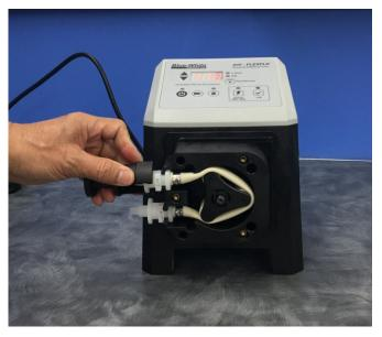
4. Place the clear cover onto the pump head. Secure the cover with the provided three thumb screws. The pump is now ready for operation.
