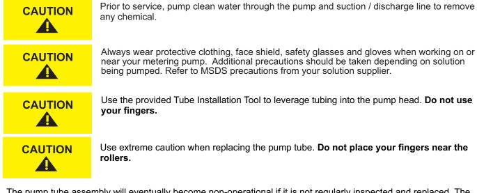
The pump tube assembly will eventually become non-operational if it is not regularly inspected and replaced. The tube life is affected by many factors, such as the type of chemical being pumped, the amount of back pressure, the motor revolutions per minute (RPM), and temperature.
