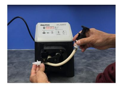
3. Stretch the tube slightly and insert the outlet (discharge) fitting into the upper retaining slot of the pump head. Pull the outlet fitting out of the pump head.
