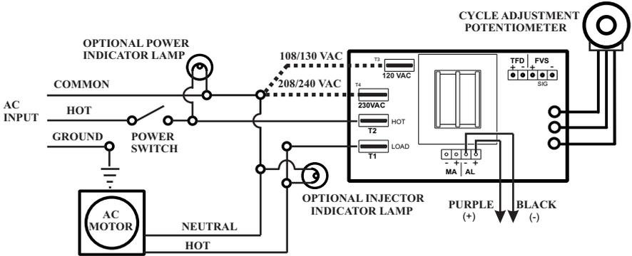
WIRING DIAGRAM - Model A-100NA & A-100NC
