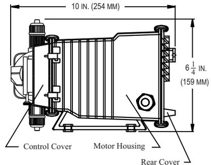
This **Shroud** is designed to weather proof this Peristaltic Pump. If the pump is wall mounted the shroud is not necessary and will still be considered weather proof.
