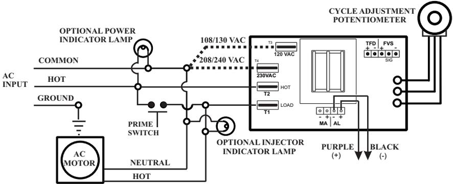
WIRING DIAGRAM - Model A-100NS
