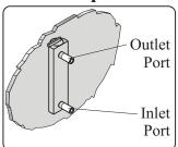
Insert the tube connection ports through the panel from the front. Hold meter firmly against the panel from front during the following step.
