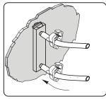
Slide the tubing over the connection ports of the meter. Once tube is in place, slide clamps against the rear of the panel so the three prongs touch the panel. Now tighten clamps, use pliers if necessary.
