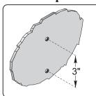
Drill two 11/32" (8.73mm) holes on 3" (76.2mm) centers on a vertical plane. Use the template on the back of this sheet if needed.
