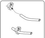
Slide the red finger clamps (P.N. 90002-206) on to tubing. Make sure to point the three prongs toward the panel.
