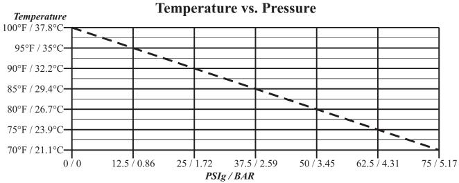
Note: The above Temperature vs. Pressure chart reflects a glued installation.
