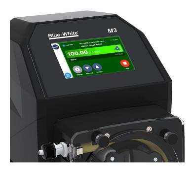
**Calibration.** Chemical metering systems should be calibrated at the initial start-up as well as after maintenance has been performed (e.g., when a tube is changed in a peristaltic pump). If the metering pump does not have an internal calibration process, operators can use a calibration cylinder and do a drawdown to check how much fluid is being pumped at a given setting. Other times, the pump can be tied to an external device such as the flow meter, which can pace the pump's output.
