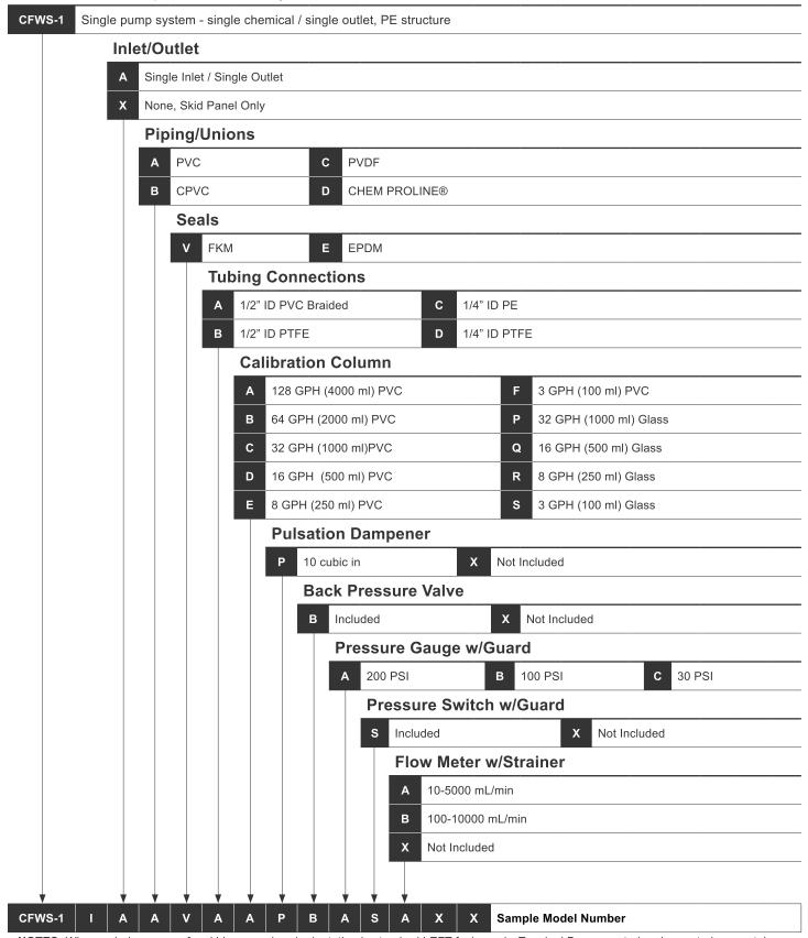
**NOTES:** When ordering pumps for skids, pump head orientation is standard LEFT facing only. Terminal Boxes quoted and mounted separately. All skids are pressure tested prior to shipment. Pumps are puchased and shipped separately.
